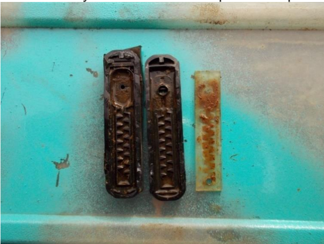
Figure 12. Dissecting and inspecting an emitter. Photo: John Harvie
