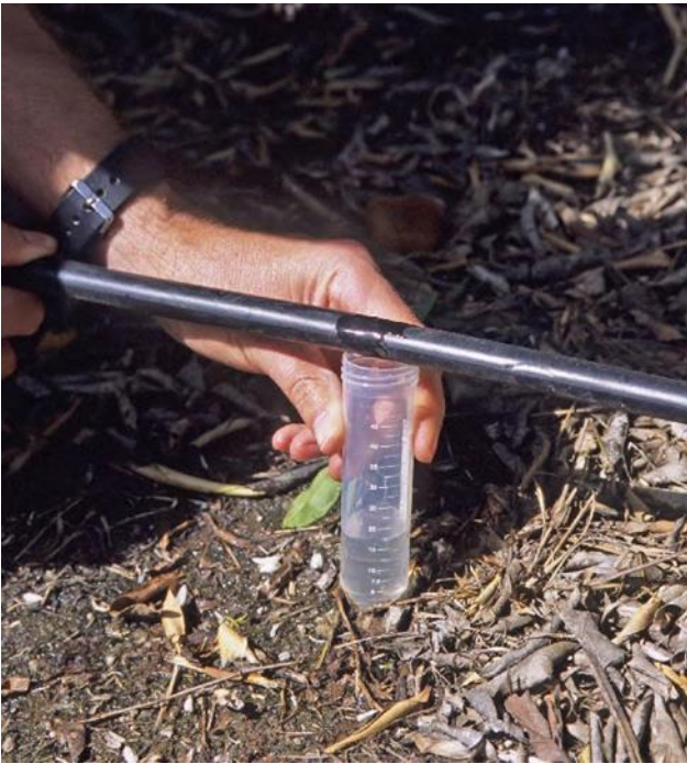
Figure 8. Measure dipper discharge rates and variation by placing containers under drippers and measuring their volumes after 36 seconds.
