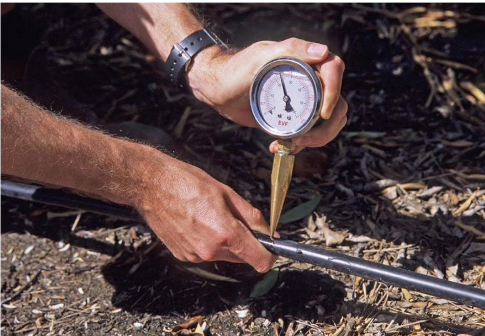
Figure 7. Using a pressure gauge and attachment
